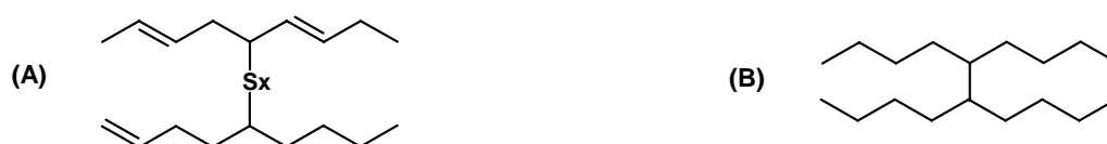
Scheme 2.3: Structures of: (A) sulfur cross-link x = 1-8 ; and (B) carbon-carbon bond created during peroxide curing
